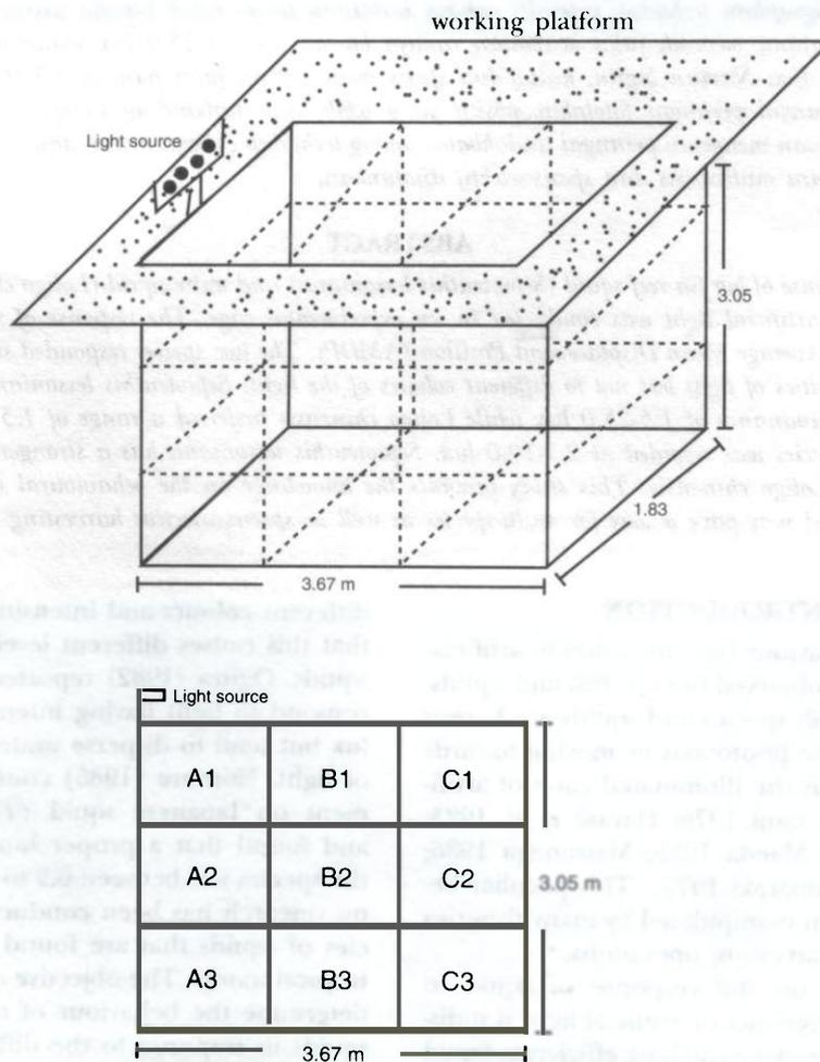
Fig 1. Configuration of the experimental cage
